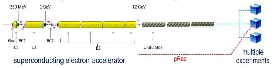
The pre-conceptual reference consists of a 12-GeV electron linac feeding a 42 keV XFEL. Located on the the LANSCE mesa it can leverage the capabilities of the existing proton/neutron facilities.
